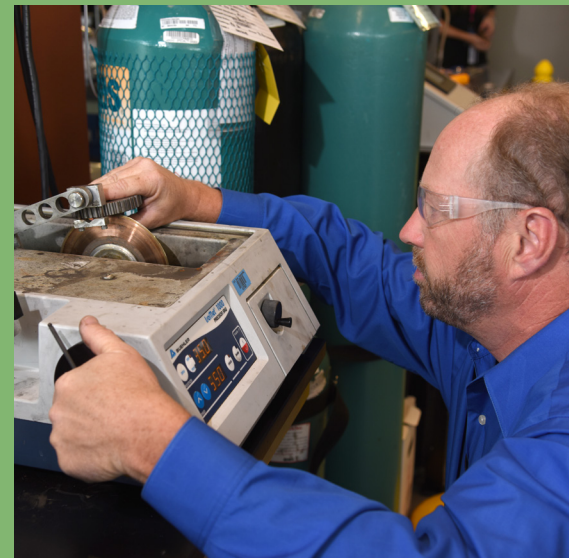
A researcher uses a medium speed sectioning saw to prepare a sample.
