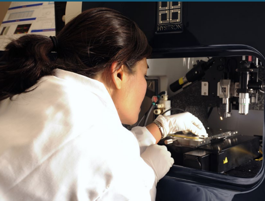
Getting a specimen ready for the Nano Indenter Atomic Force Microscope.
