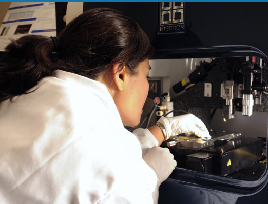
Getting a specimen ready for the Nano Indenter Atomic Force Microscope.
